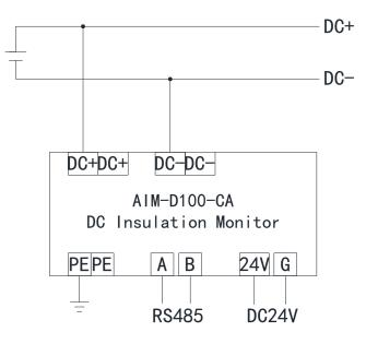
The AIM-D100-CAI DC Insulation Monitor is wired as shown in the following schematic when monitoring the DC system:
