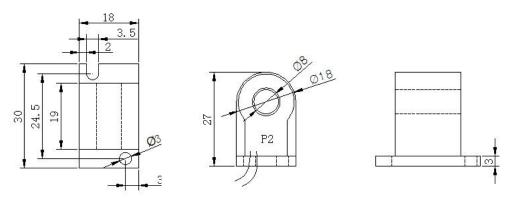
Note: The primary current enters from P1 and exits from P2 (glue filling surface). The red and yellow lead lines are S1 and S2. The length of the lead line is  $2m \pm 10$  cm.
