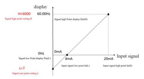
Setting: H: 6000,fiWe can get L according to the chart: (In (H)-In (L))/In (L) = (Dis (H)-Dis (L))/(Dis (L)-L). So L = 0 - (6000-0) \* 4 / (20 - 4) = -1500.
