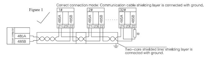
Recommendation of adding matched resistance between A ,B of the last meter,the rated resistance range is  $120\Omega\sim10k\Omega$ .
