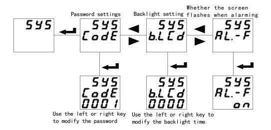
Enter the programming menu, press left or right key to select the LCd page, press Enter key to enter revising condition, left or right key to modify the time to  $000 \sim 255$ s. To LED display meter, this item is invalid.
