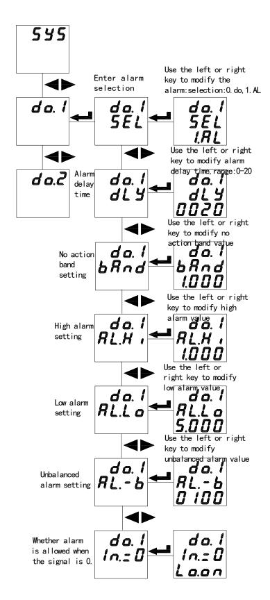
Note: 1. No action band setting, high alarm value setting and low alarm value setting correspond to the display value of the meter, and the value contains a decimal point. Example: Input 100A/5A,100% current high alarm,95% return; 20% current low alarm,25% return,"AL.Hi"taken as 100.0,"AL.Lo"taken as 020.0,"bAnd"taken as 005.0;
