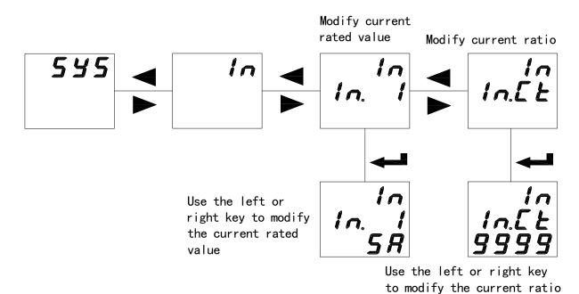
Note: IN.I is the current rated value ,IN.U is the input voltage rated value; IN.CT is the current ratio,and IN.PT is the voltage ratio.
