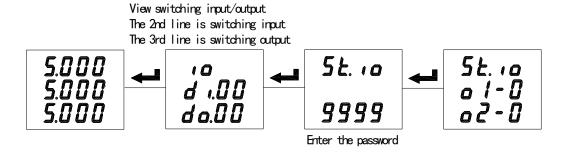
View the switching status of AMC72/96(L) single-phase current meter(same single-phase voltage meter):
