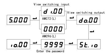
The liquid crystal (LCD) display meter has a switching input/output indication under normal measuring condition, without pressing the shortcut key to look over.
