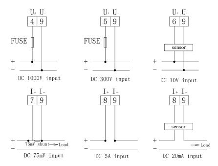
Note:1. The symbol "\*" indicates current input terminal, this wiring is for reference only , the specific wiring diagram on the meter prevail;
