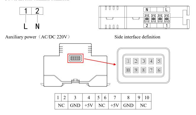
The side interface is used for the AWT100 wireless communication terminal to supply power through the AWT100-POW power module AC220V. The AWT100 wireless communication terminal is connected to the AWT100-POW power supply module through pins and fixed together by a buckle. The connection diagram is shown in Figure 4:
