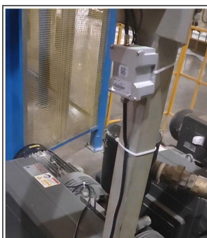
Installation Picture of ATE300P installed on Motor Shell
