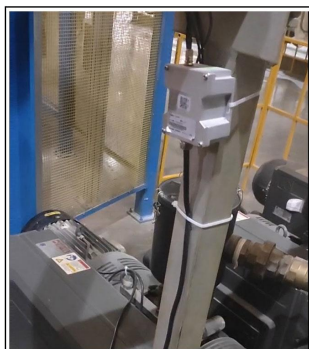
Installation Picture of ATE300P installed on Motor Shell
